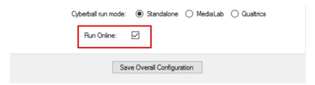
With Run Online option checked, the "Online/Web" tab, seen here, becomes enabled. The "Run Online" on the "Basic" screen must be checked to work fully with the online version of Cyberball through the Cyberball configuration application.
